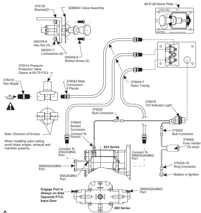
**WARNING:** Connect directly to the air supply. Do not use tubing between the air supply and the pressure protection valve.
